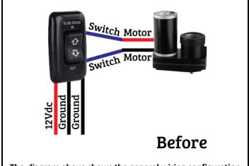
The diagram above shows the general wiring configuration of the slide unit in your RV prior to installing the Smart RV JAS30 Remote Control.
