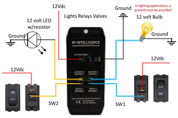
\*Connecting an external Switch Switch can use the same 12Vdc as the module \*\*Relays and Valves connect the same
